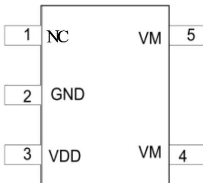
Figure 2. Pin Configuration
